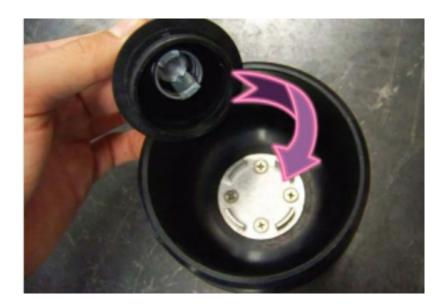
To install the post, center the post on the mounting flange in your new Rennline Oil Filter Housing and press firmly. The post will snap into place when seated properly and spin freely. Your Rennline Billet Oil Filter Housing is now ready for installation. Refer to factory Porsche manuals for the appropriate oil filter and gasket specifications.
