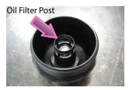
Start this installation by removing the oil filter post from the factory oil filter housing. This post allows adequate flow from the filter housing into the crank case and is required on your new Rennline filter housing. To remove the post push the top of the post towards the outer rim of the housing. The post will make an audible pop when it is disengaged from the base.
